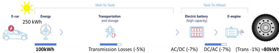
Figure 5-2: Energy efficiency of a battery electric vehicle
