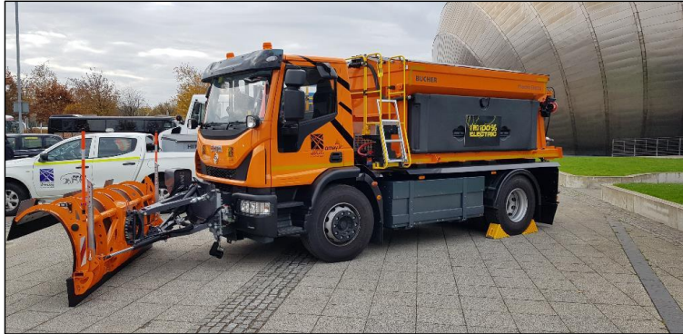
Figure 11-2: Electra Gritter developed for Transport Scotland for use on the Forth Bridges
