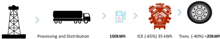
Figure 5-1: Energy efficiency of an internal combustion engine vehicle
